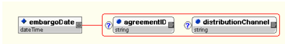
Figure 3.10 Embargo Date structure
